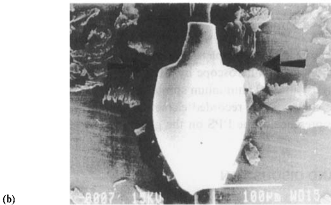
FIGURE 1 PPS microdroplet formed on a E-glass fiber: (a) before debonding; (b) after debonding.
